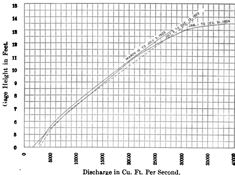
Fig. 46.—Rating Curves, Wisconsin River at Necedah, Wis., Showing Changes in Head Due to Changes in Cross Section.
