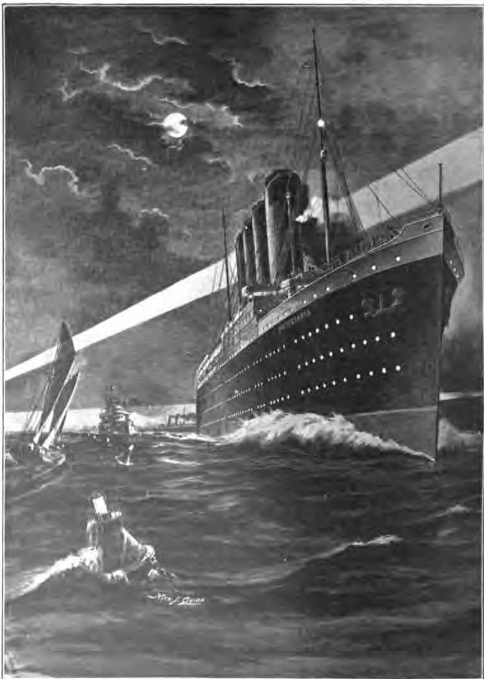
Fig. 36. Cunard Line Steamship Mauretania . Built in 1907 at the yards of Swan, Hunter & Wigham Richardson, Wallsend-on-Tyne, England. Largest ship afloat. Length 790 ft. (5 ft. greater than that of her sister ship the Lusitania ); width, 88 ft.; depth 60 ft. 6 in.; engine horse-power, 70,000; displacement, 46,640 tons. The vessel is here shown making her way to sea at night from New York Harbor along new Ambrose Channel, guided by light-buoys.
