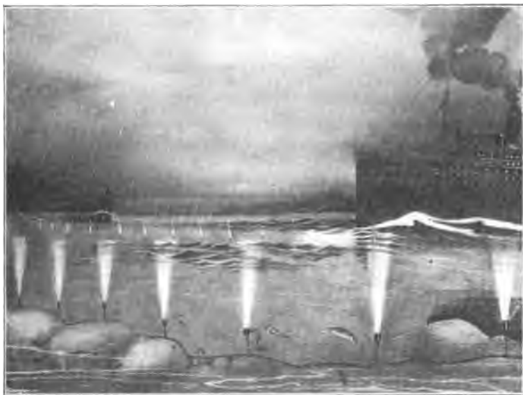
Fig. 37. "Subaqueous" System of Harbor Lighting. Invention of Mr. Leon Dion, of Wilkesbarre, Pa. Incandescent lamps, with reflectors designed to concentrate the light into parallel beams, are connected at intervals to a cable conductor fed from a generator on shore.
