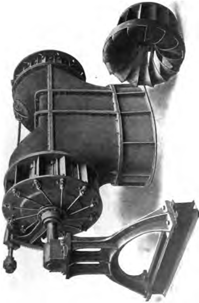
Fig. 104. Two Risdon-Alcott Turbines Mounted on Same Horizontal Shaft, Fitted with Balanced Hinged Gates, Discharging Centrally Into Common Draft-Tube.
