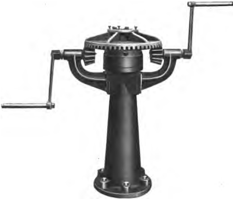
Fig. 128. Head-Gate Hoist for Operating Gates under Pressure. Upper end of gate stem is threaded to match a bronze nut attached to bevel gear shown in cut. Ball bearings are used to insure easy operation. Dayton Globe Iron Works Co., Dayton, O.
