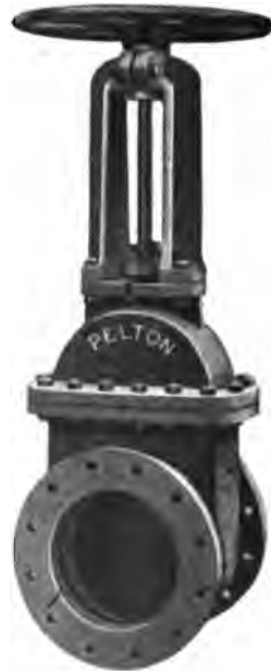
Fig. 111. Straightway Valve of Single-Disc Type, with Rising Spindle, Intended for Pressure on One Side Only. Disc rises clear of opening, giving a perfectly free way for the water. Seats are of bronze, to be replaced when worn.
