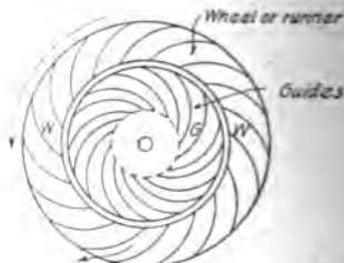
Fig. 69. Fourneyron Turbine, Radial outward flow.
