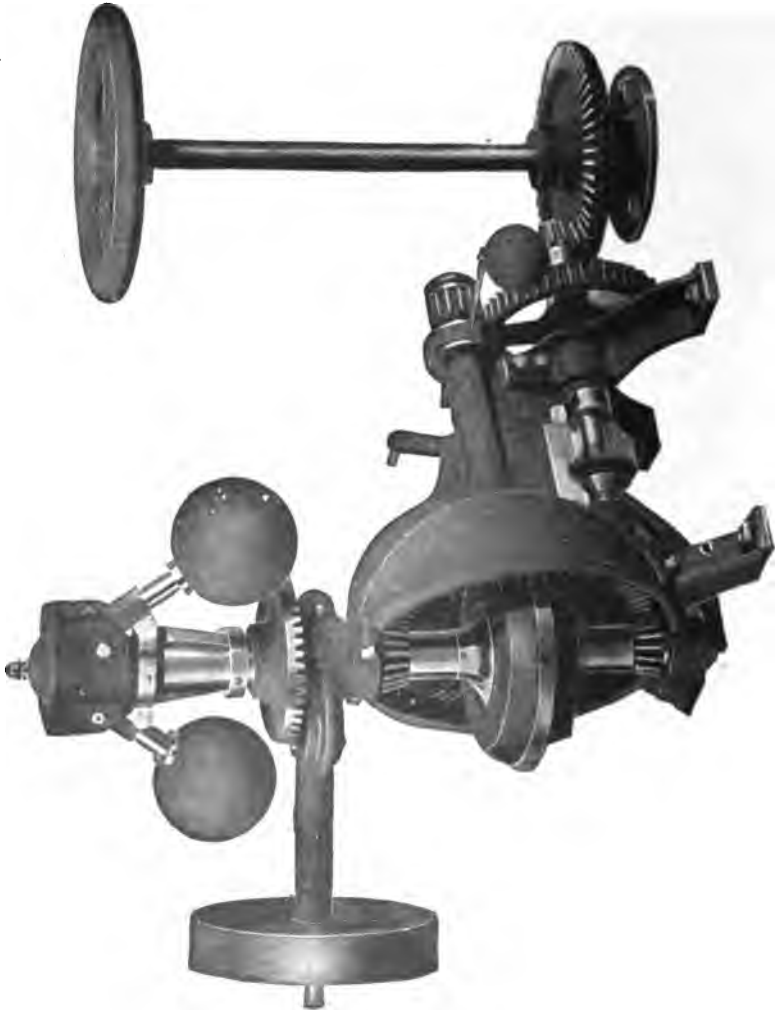
Fig. 122. Standard Type "Woodward" Governor, Suitable for General Mill Work.
