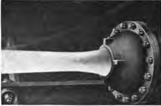
Fig. 50. Stream of Water from Pelton Needle Nozzle Operating under 300-Foot Head and Developing 1,500 H.P.
