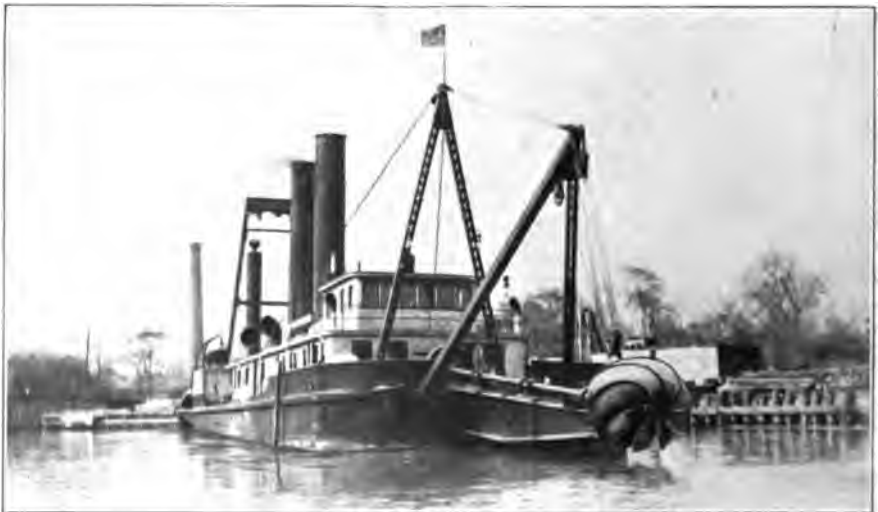
SUCTION DREDGE "FRANCIS T. SIMMONS." Engaged in hydraulic filling operations for the park system of Chicago. Capacity, 1,500 cubic yards an hour.
