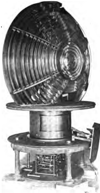
Fig. 57. Third-Order Lightning Light, Toledo (Ohio) Harbor. Fresnel lenticular apparatus, showing clockwork for revolving.
