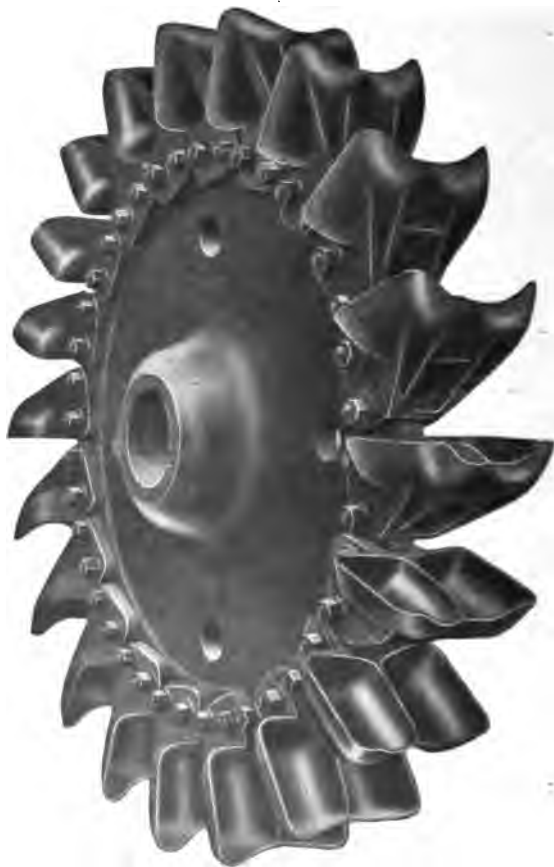
Fig. 42. A 5,000-H.P. Pelton Water-Wheel Runner. This wheel, 9 ft. 10 in. in diameter, is capable of developing 5,000 h.p. at 325 r.p.m. under 865 feet of effective head.
