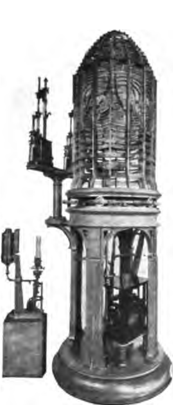
Fig. 56. Light for Lighthouse on Cape Villano, Spain. Showing apparatus giving double flash every 15 seconds.
