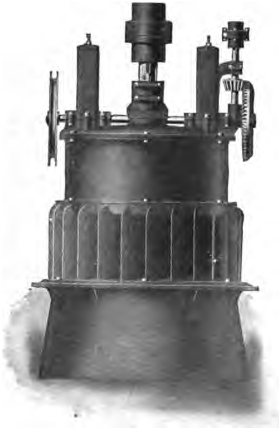
Fig. 106. Smith Turbine with Cylinder Regulating Gate Fully Raised. Courtesy of S. Morgan Smith Co., York, Pa.
